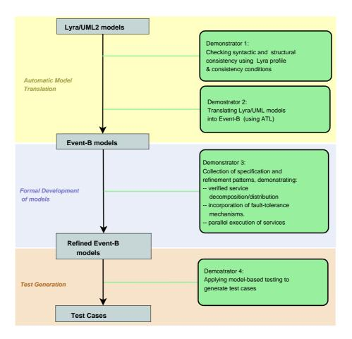
Fig. 2.1: Tool chain for Lyra-B integration and demonstrators
