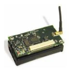
Each user carries a smart dust mote (with a unique id, so the mote acts as a badge, sort of speak) and a PDA as an interaction device. Each room is equipped with a smart dust base-station (receiver), which is connected to a controller application. The latter uses the CAMA middleware to communicate with the PDAs through Wi-Fi. When a user enters a particular room, his/her PDA shows the relevant information and/or services available for that room.
